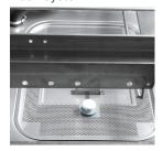
In addition, they include one filter for separating the water in the tank from the dirt, an one filter shaped like a tray, which can be easily removed and cleaned. Optional steam condenser.
