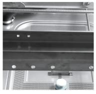
In addition, they include one filter for separating the water in the tank from the dirt, an one filter shaped like a tray, which can be easily removed and cleaned. Optional steam condenser.
